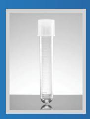
17x100mm, 14 mL polystyrene round bottom test tubes have a 1,400 RCF rating. The tubes come with polyethylene dual-position snap caps, which offer both vented and fully closed positions. RNase/DNase-free.
